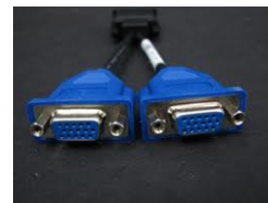
d - Y-Cable to split monitor signal
