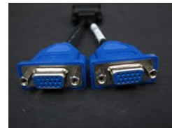
b - Y-Cable to split monitor signal
